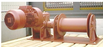
mooring winch with automatic and manual free running
